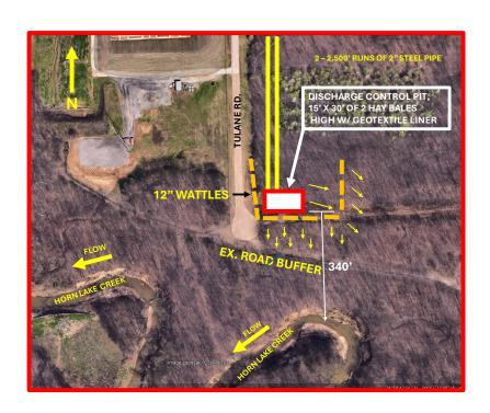
**DISCHARGE CONTROL/FILTERING DETAIL**
