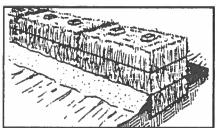
trenched a minimum of four inches and anchored with two stakes driven toward the previously laid bale. Straw bales that are not buried are improperly installed, have no useful function, are a waste of money, and could result in substantial fines.
