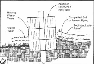
s between bales shall be wedged with straw. Loose straw scattered immediately uphill increases barrier efficiency. Under no circumstances should straw A higher than B
