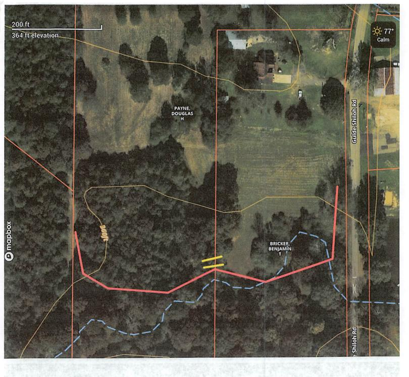
Red line would be the silt fence and future levee. The two yellow line would be where the haybales would be placed. Levee design
